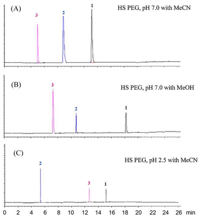
**Fig. 3.** Chromatograms illustrating the effect of changing the pH value and the organic modifier on the selectivity. (A) HS PEG, pH 7.0 with MeCN, (B) HS PEG, pH 7.0 with MeOH and (C) HS PEG, pH 2.5 with MeCN. Representative compounds are: (1) phenanthrene, (2) prometryn and (3) ibuprofen.
