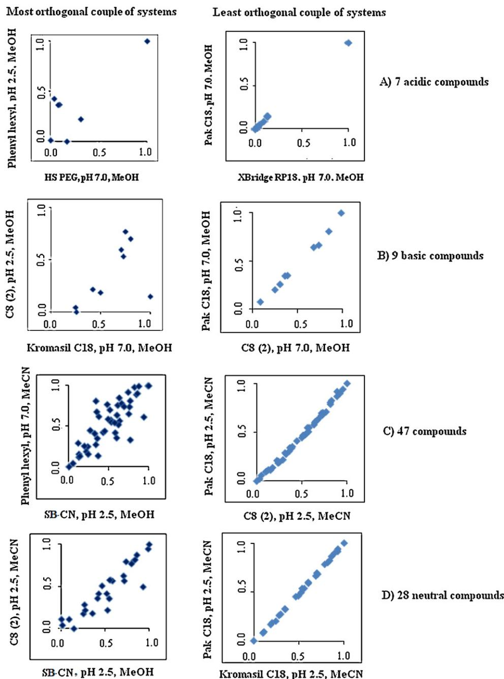
**Fig. 7.** 2D plots representing the most (left) and the least (right) orthogonal couple of system with the subsets of probe solutes: (A) 7 acidic, (B) 9 basic and (C) 47 solutes include 28 neutral solutes in (D). The coordinates of each compound in a plot are its normalized retention times in the two systems.
