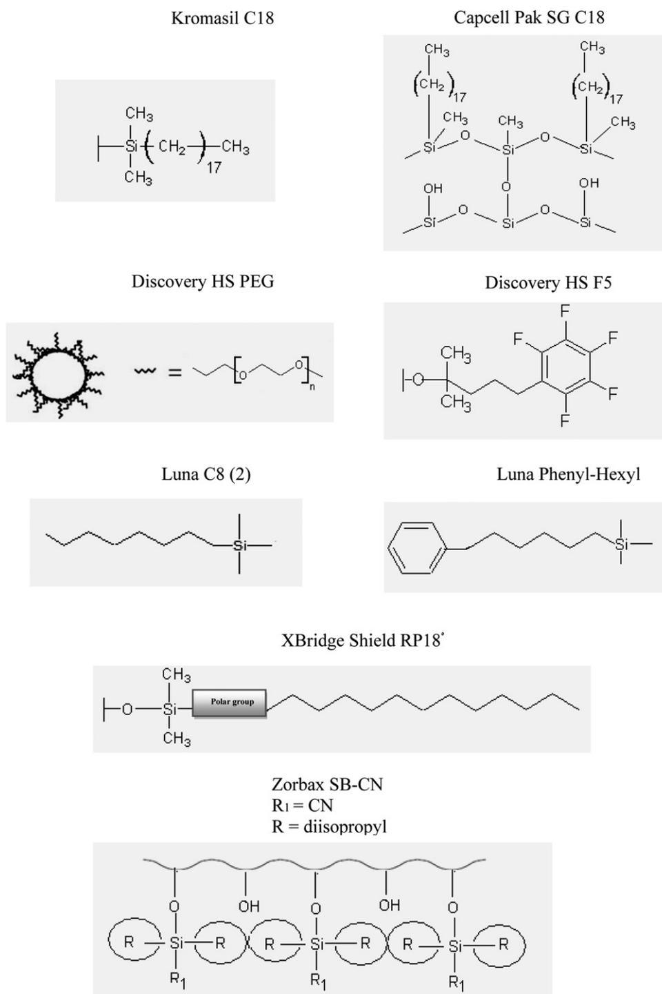
**Fig. 1.** Structures of the different stationary phases.
